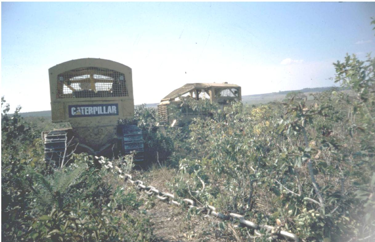
**Figure 2.3: Clearing of native cerrado vegetation with the correntão chain system**
